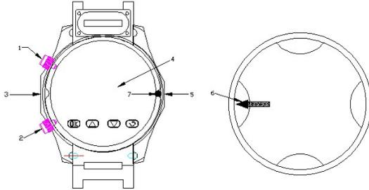
1: on / off button 2: OK key 3: USB interface 4: Touch Screen 5: Camera 6: back cover arrowhead mark(point to camera is turn on,30 degree is turn off) 7 : back cover contraposition
